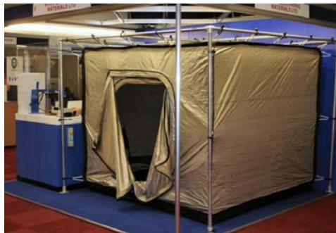
An example of a low-cost shielded tent (courtesy of Hitek Electronic Materials Ltd)
