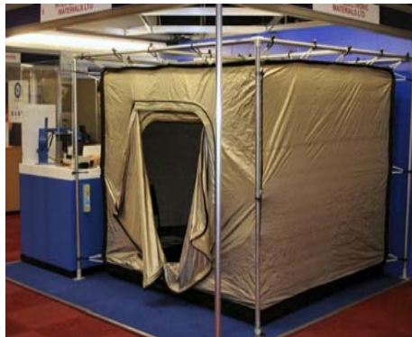
An example of a low-cost shielded tent (courtesy of Hitek Electronic Materials Ltd)
