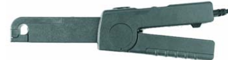
Tektronix A622 Current Probe 0.05 to 100A @ 10 or 100mV/A DC - 100kHz BNC or twin banana plug output
