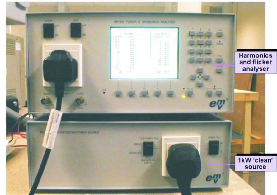
A commercially-available harmonics analyser, with mains source (Courtesy of AD Compliance Services Ltd)
