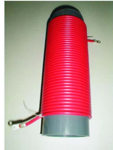
An example of 50μH inductor under construction for a home-made LISN
