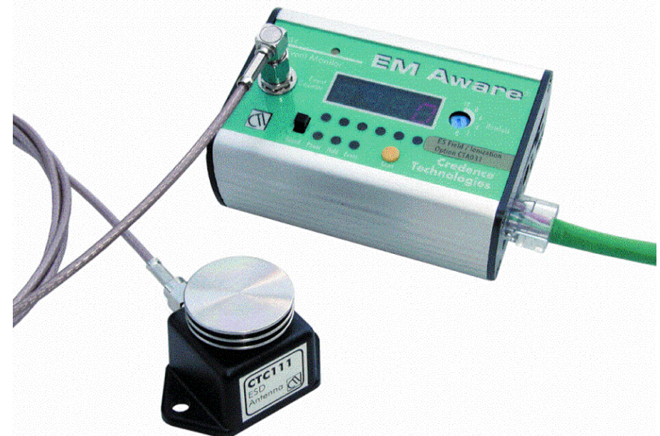
Example of an ESD event detector (courtesy of Credence Technologies, Inc.)
