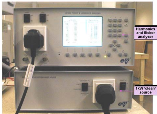
Figure 24 A low-cost harmonics analyser, with a 1kW sinewave source
