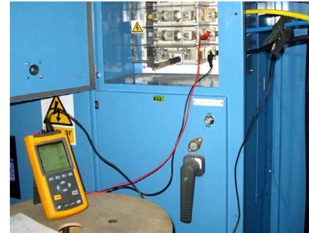
Figure 12 Typical harmonic current measurements in the road tunnel lighting scheme
