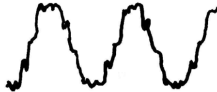
Figure 21 An example of a domestic mains waveform in Israel, in 2000
