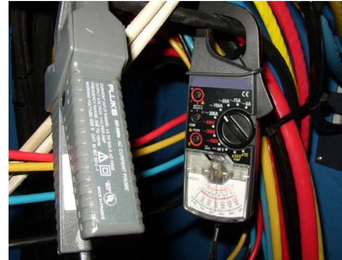
Figure 13 Comparing a True-RMS ammeter with an ordinary electricians clamp-on ammeter
