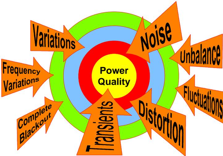
The diagram on the left is an attempt to show, in diagrammatic form, the various EMC phenomena that can influence power quality, where the network is highly reliable (conforms to EN 50160:2000 Voltage characteristics of electricity supplied by public distribution systems).
