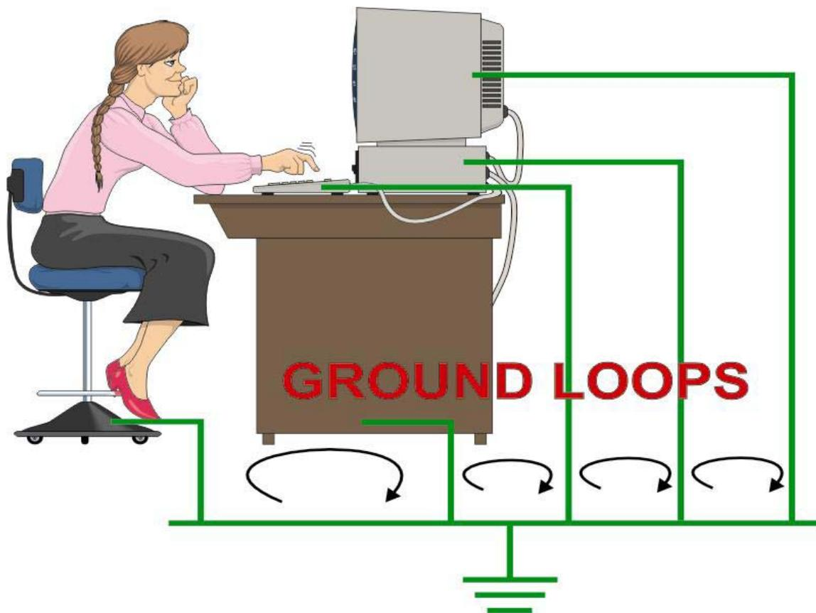
The electrical characteristics of these earth paths or ground loops will differ greatly; consequently voltages may be developed in the earth as a result of small leakage currents which tend to exist in electrical/electronic equipment. Coupled with this, these ground loops can act as antennae picking up high frequency interference. Typical problems associated with groundloops are 'humming' from audio equipment and vertical bars on CCTV screens.
