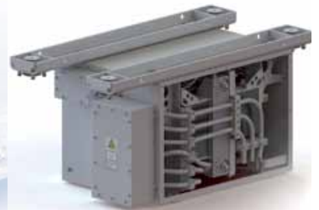
REO absorption circuit choke: Absorption circuit inductor for a multi-system vehicle (25 kV, 50 Hz AC mains, 5 kV, 16.7 Hz AC mains, 3 kV DC mains, 1.5 kV DC mains) The inductor is employed in combination with a capacitor in the cooling system of the converter container to create a resonant circuit for a specific resonant frequency. The robust construction is designed for secure assembly, with special damping elements absorbing vibrations.
