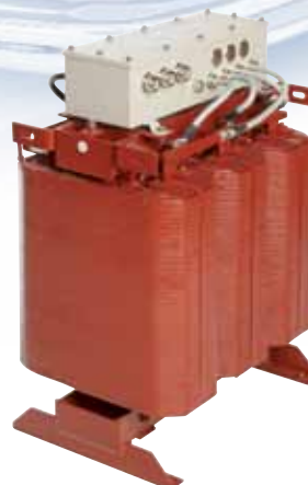
REO three-phase converter transformer – is employed in auxiliary converters for the galvanic separation of link DC voltage up to 2000 V DC. Special impregnation serves to protect the transformer against external influencing factors.
