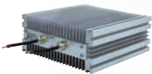
REO damping resistor The NTT R 159 resistor is used as a damping resistor in series with a filter capacitor in a traction power converter on the 3-kV DC mains.
