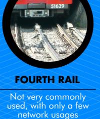
Underground. The extra rail carries the electrical return, meaning that the running rails don't carry any current.
