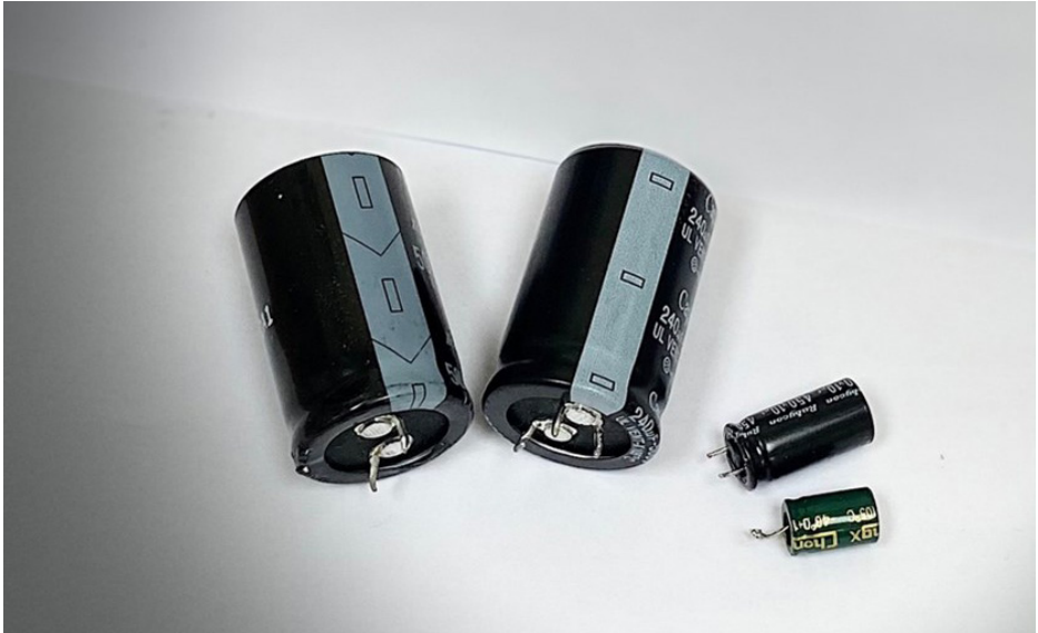
Figure 13 Electrolytic capacitors are used as a prime energy storage device
