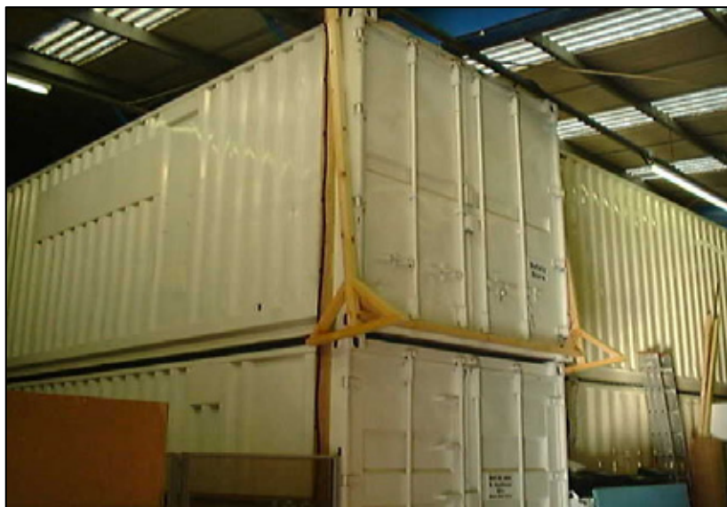
Figure 75 Examples of stacked shipping containers used as shielded EM Zones
