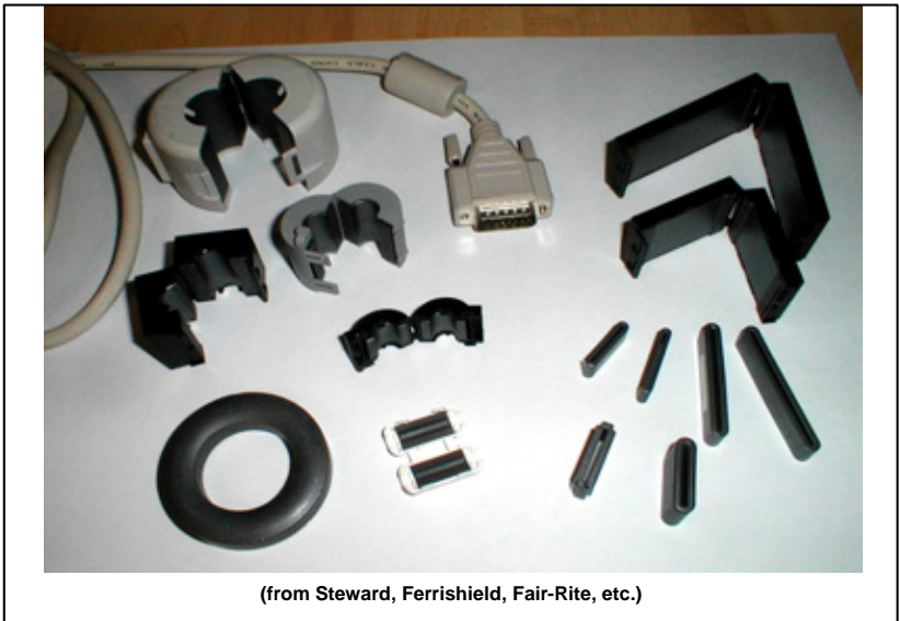
Figure 58 Examples of ferrite suppressers for CM cable currents
