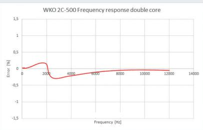
Figure 4: Double core frequency response
