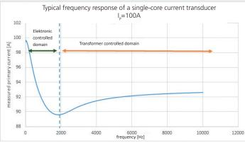
Figure 2: The peformance of the electronic and transformer stages are not balanced.
