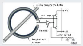
Figure 1: Closed loop compensated current transducer principle
